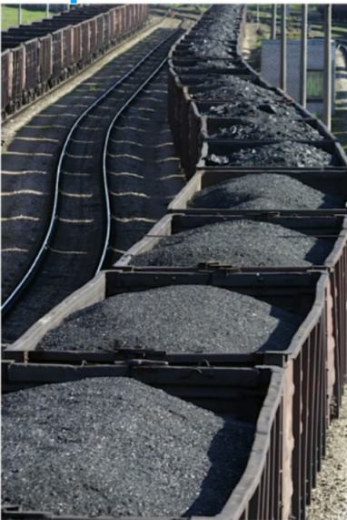
Figure 4: Fuel for 1 GW plant for one day. The coal plant’s fuel requires a 70 car train. The nuclear plant’s fuel fits in a two gallon jug. Newcastle 6700 is a good coal. Most coal’s are worse.
