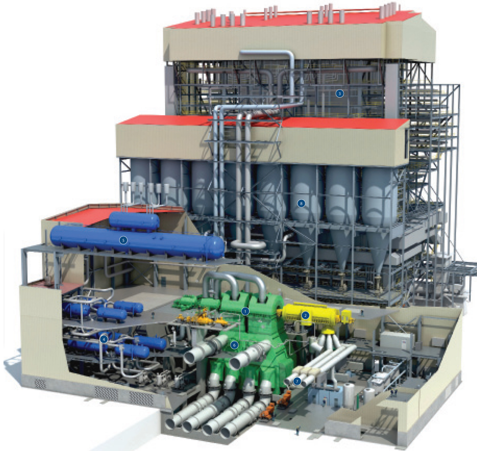
Figure 9.1: Manjung 4, A Modern 1 GW electric coal plant. Turbine(green) in the foreground. Boiler in the background.
