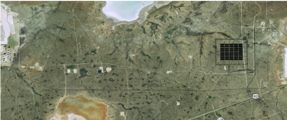
Figure 3.8: Satellite view of the Hi-Store facility. If the US were to go all nuclear, the 20 pads on the right would handle at least 12 years worth of used fuel.
